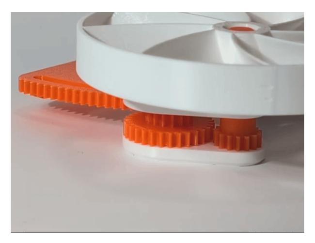
The big gear immediatly disenganges the small gear as soon as there is no more torque on it.
